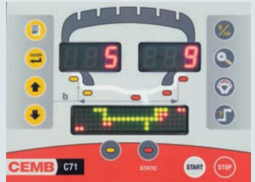
Counterweight position set-up.
