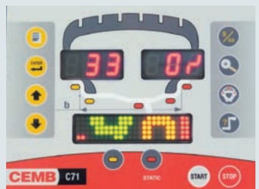
Optimization of rim-tyre position.
