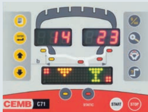
Position repeater display for internal counterweight application.
